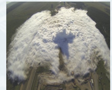
CO 2 cloud from a rupture test performed at DNV GL Spade Adam / Image: DNV GL
